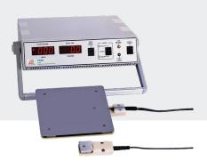
The Trek® 156A tests the efficiency of an ionizer's ion production by timing how long it takes air ions produced to discharge a floating plate that has been pre-charged to either a positive or negative value. The Trek 156A also tests the balance between positive and negative air ions by measuring the offset voltage generated on a floating plate due to an imbalance of positive and negative air ions impinging on the plate from the ionizer.
