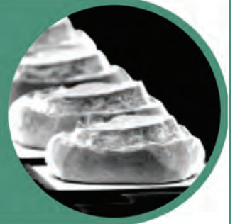
FIGURE 2 SEM image of a mechanically applied gold stud bump
