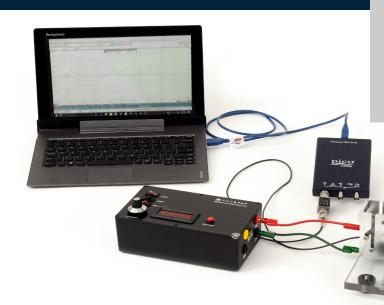
Electrostatic Shielding Bag Testing per ANSI/ESD STM11.31 and IEC 61340-4-8.
