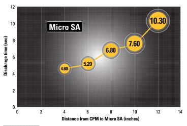
Results are for a static charge reduction of 1000-100V; 17 lpm air flow into Micro SA. Testing in accordance with ionization standard ANSI/ESD STM3 1-2006 of the ESD Association. Results may vary depending upon application and environment.
