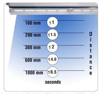
Measured using Simco-Ion CPM Model 280A w/HEPA flow (60 fpm or 0.3m/sec) & CDA flow @ 2.5 l/m/n.
