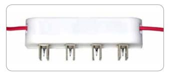
Simco-lon's IsoStat technology is the first balancing technology for ionizers to guarantee intrinsically balanced ionization and elimination of complicated feedback circuits. IsoStat is based on a law of physics, Conservation of Charge, which states that charge cannot be created or destroyed in an isolated system. By isolating the ionizer's emitter points from ground, IsoStat ensures equal numbers of positive and negative ions. Characteristics of IsoStat ionizers include:
