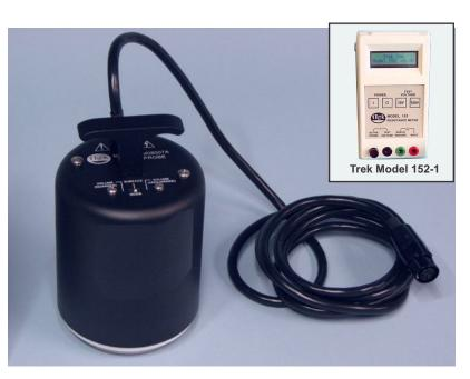
The Trek Model 152P-CR-1 Concentric Ring Probe is capable of measuring surface and volume resistance in materials as per IEC or ESDA standards. A three (3) position switch on the probe selects surface resistance or volume resistance measurements with either a guarded or unguarded outer electrode. (See page 2.)
