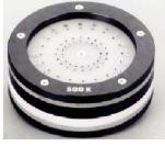
Surface Resistance Calibration Test Fixture
