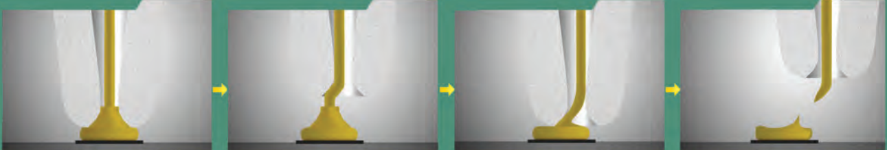
FIGURE 1 : Schematic of stud bond using software modification on ball / wedge bonding machine
