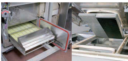
Inlet Condensation Trap
