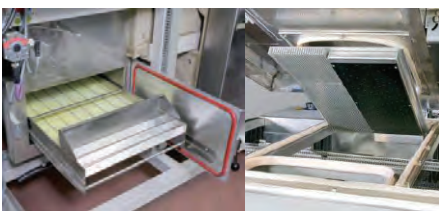
Inlet Condensation Trap
