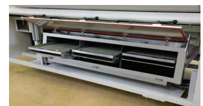
Modular Cooling Zone
