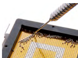
Easy distribution of solder balls on a universal mask
