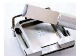
Squeegee applied solder paste
